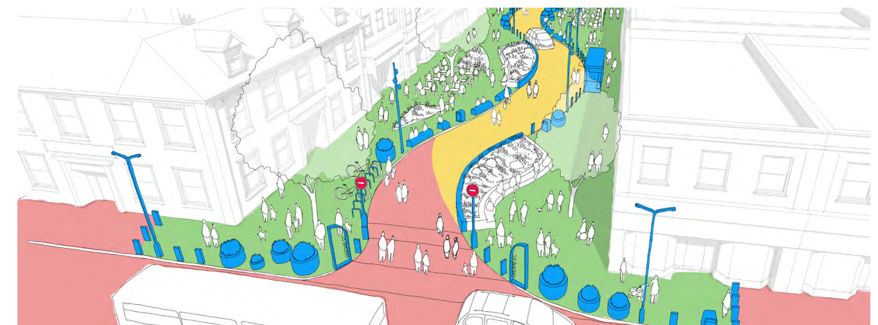
(d) Traffic calming methods - The application of horizontal deflections (e.g. bends and chicanes) that are enforced by VSBs will limit hostile vehicle speeds. Reducing hostile vehicle speeds significantly reduces the severity of a vehicle-borne attack with fewer casualties in a VAW attack on people and less damage from a penetrative vehicle impact on other assets. Reducing vehicle speeds can reduce the requirements and associated costs of HVM measures and provide more opportunities to deploy discreetly integrated protection.
