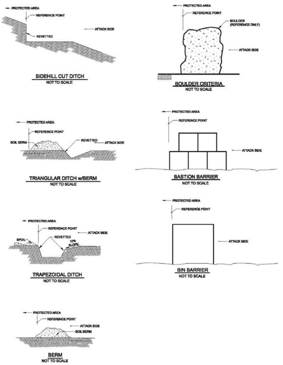
FIG. A1.1 Vehicle Barrier Reference Points
