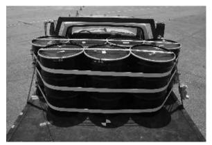
FIG. 2 Typical Ballast Attachment, Rear View
