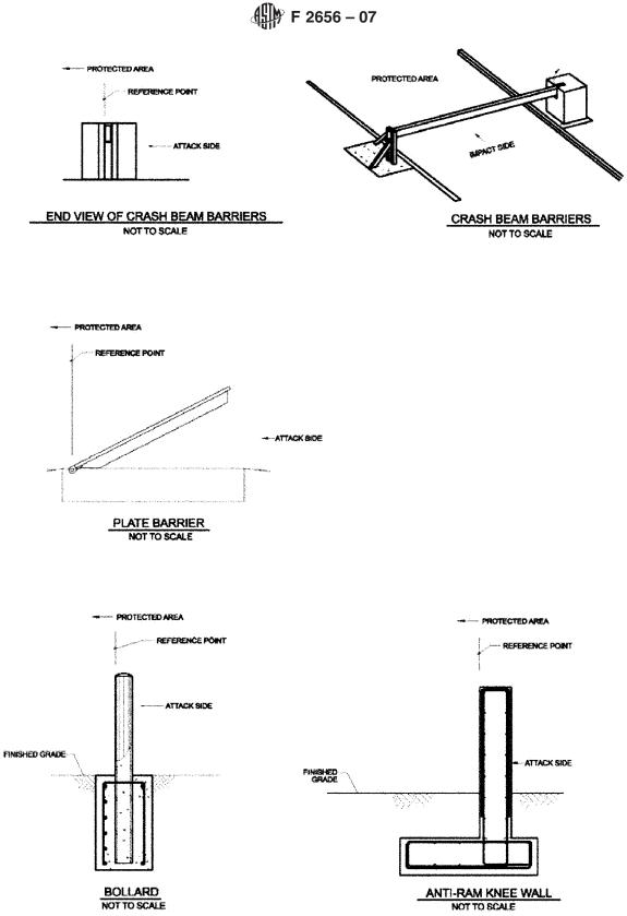
FIG. A1.2 Vehicle Barrier Reference Points
